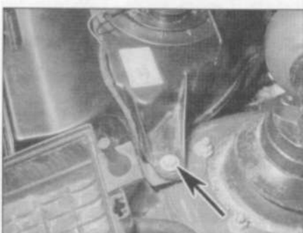
6.6a Hydraulic fluid reservoir securing screw . . .
