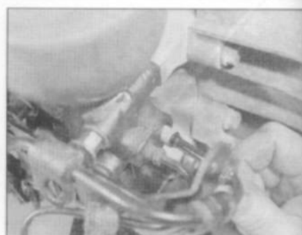
5.9 Use new seals when reconnecting the fluid pipes
