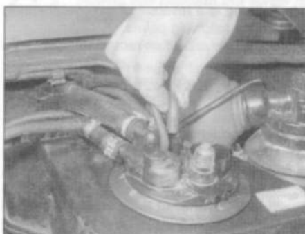
6.3b . . . and pull the fluid return hoses from the reservoir centre section
