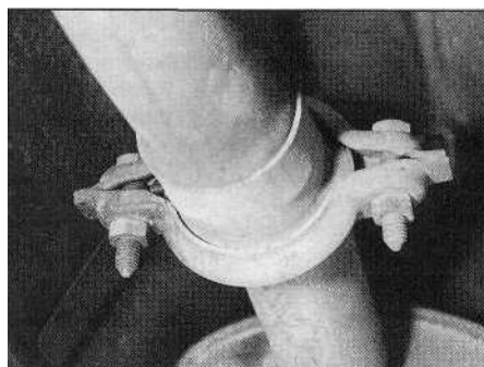
18.10 Typical exhaust system clamping ring
